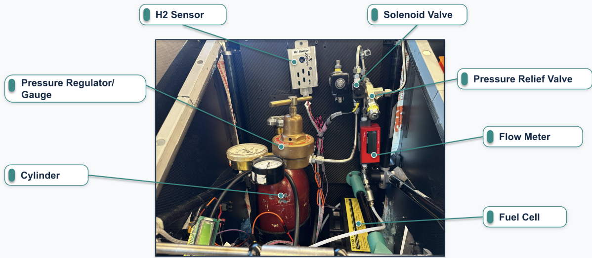
Figure 2: Diagram of Hydrogen System in Vehicle
