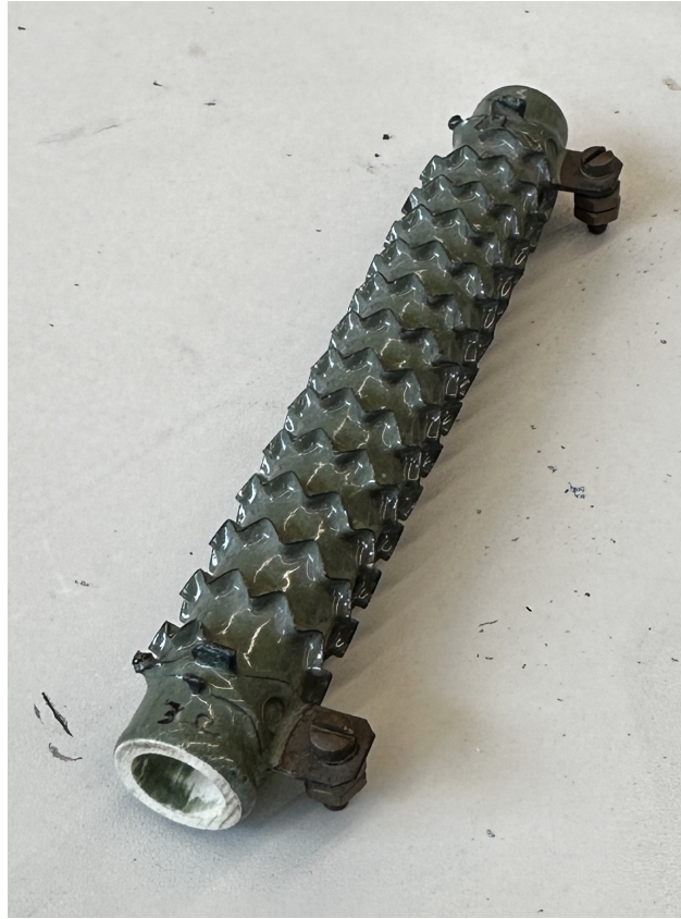
Figure 7: Resistor for Discharging Capacitor
